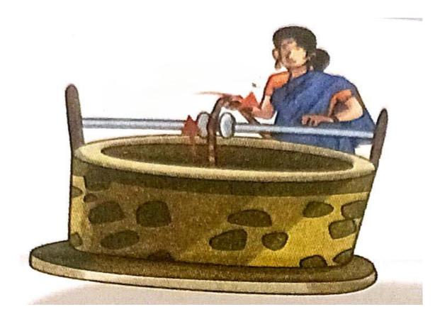
In the figure load is to be lifted in upward direction and the rope is pulled in the downward direction .So by changing the direction of force it becomes easier to lift a bucket of water.
