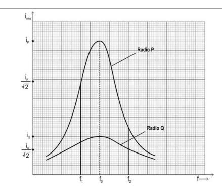
(a) Which radio will allow a person to hear a radio channel of frequency fo, without the interference of other frequencies? Give reason.
