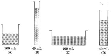
Volume of water in each vessel is shown above. Arrange them in order of decreasing pressure at the base of each vessel. Explain the reason.
