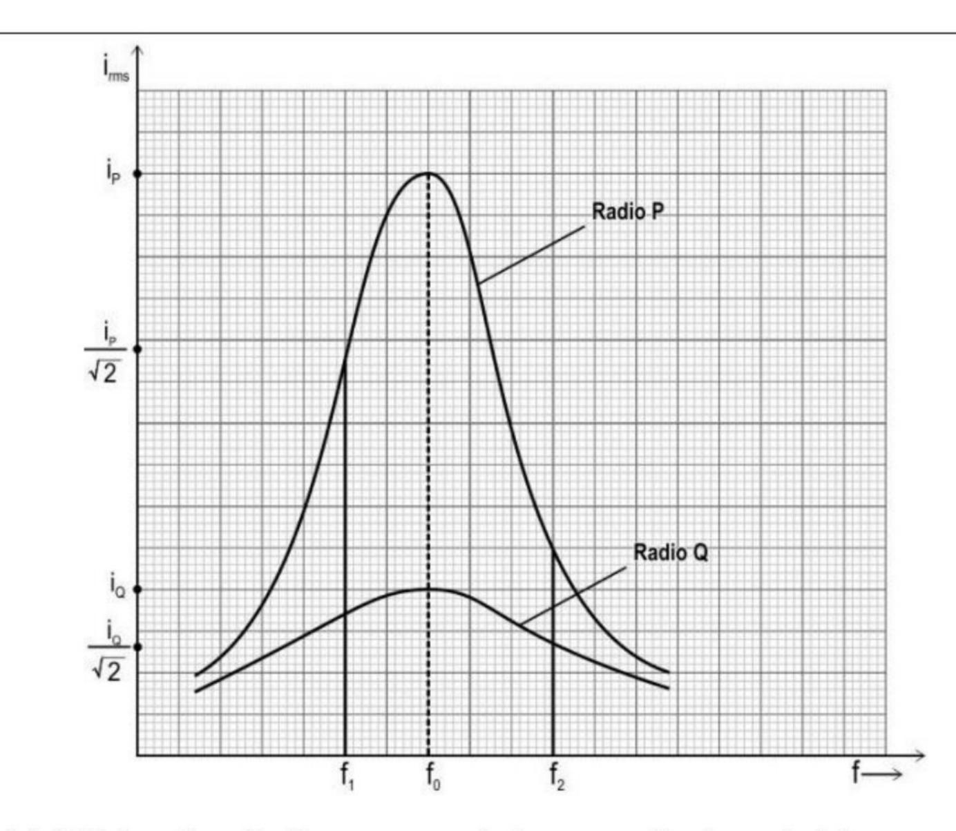
(a) Which radio will allow a person to hear a radio channel of frequency  $f_{\text{o}}$ , without the interference of other frequencies? Give reason.
